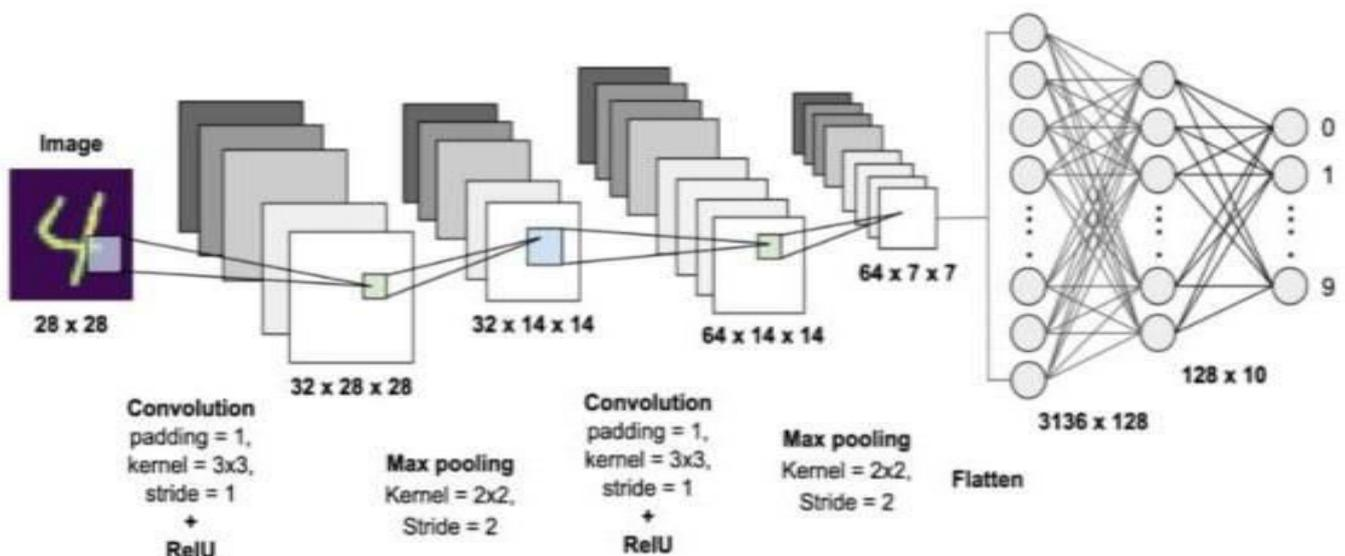
Fig 2 :CNN Architecture
